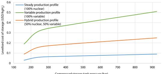
Figure 2.9: Levelised cost of hydrogen storage for different compressed tank pressures
