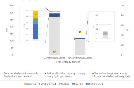
These results demonstrate that the case of nuclear power is further improved when the system requires large amounts of baseload hydrogen at high carbon constraints, as long as the hydrogen storage infrastructure is not available and/or storage costs remain high. In such conditions, the following generic conclusions for integrated electricity and hydrogen production systems can be drawn:
