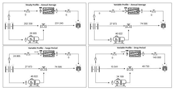
Figure 2.5: Average "seasonal" hydrogen flow for variable and steady production profiles
