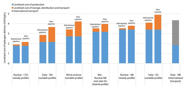
The "expanded large-scale hub" configuration highlights the decisive impact of pipeline lengths on the LCOHD. Although the hydrogen production plant is of 1 000 MWe, the benefits of the large scale are offset by the greater distances. This holds particularly true for the variable profile systems, which see their delivery costs rising faster than those of other production profiles.
