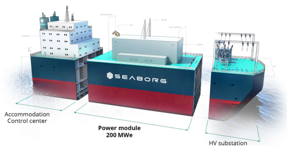
200MWe Power Module of the CMSR Power Barge
