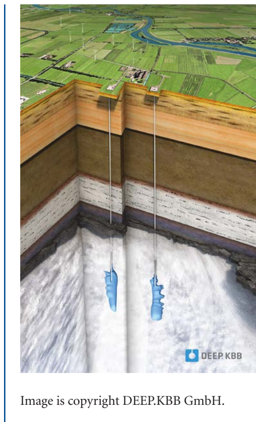
Figure 5.5 Stylized representation of underground salt cavern
