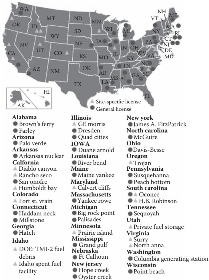
FIGURE 10.6 Locations and types of independent spent fuel storage installations (ISFSIs).
