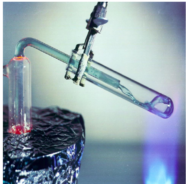
Figure 3-1: Images of novel nuclear fuel physical forms. Left – cross section of TRISO fuel, showing <math><1\text{ mm}</math> kernels fissile material surrounded by layers of graphite and silicon carbide, dispersed within a graphite matrix [34]. Right – molten lithium beryllium salt of the type under consideration for use in many Molten Salt Reactor (MSR) designs [35].
