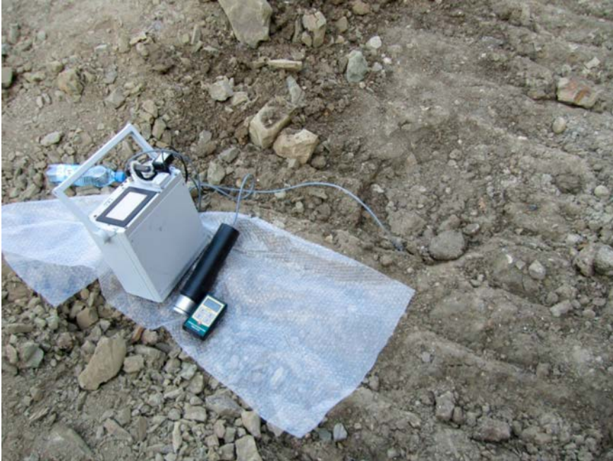
FIG. 6. The A 2 M 4000 monitor for measuring radon and thoron activity concentration in soil gas together with the gamma dose rate.
