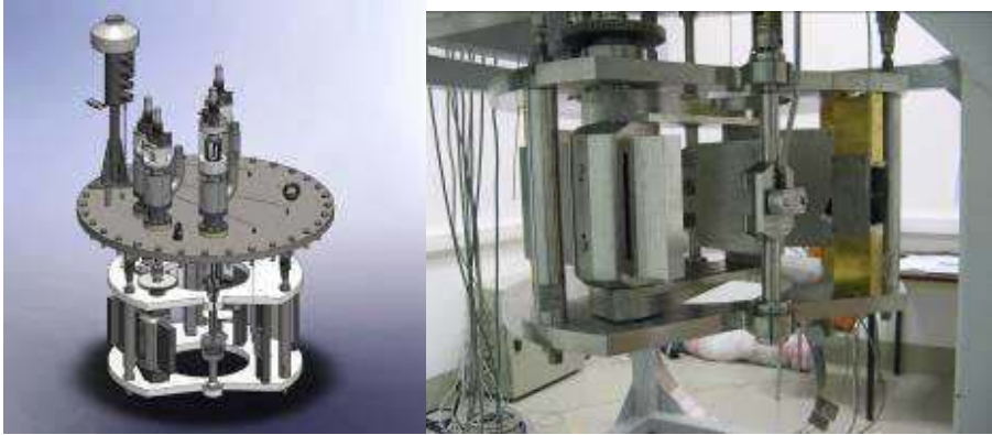
FIG. 9. MULTIREFLECTOR mock-up devoted to in-sodium ultrasonic telemetry study.
