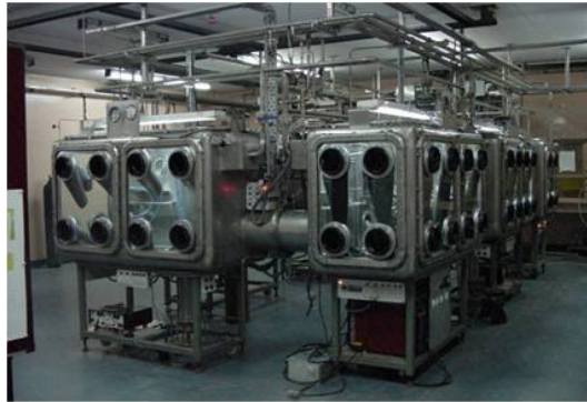
FIG. 7. View of the facility for fabrication of sodium bonded fuel pins.
