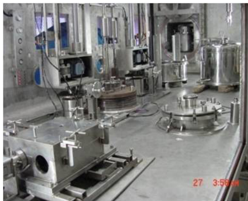
FIG. 8. View of the electrorefiner and other equipment inside inert atmosphere glovebox.
