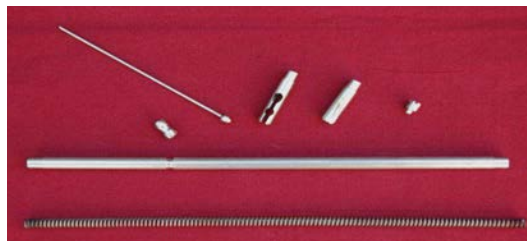
FIG. 17. MOX fuel pin components.
