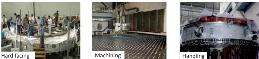
FIG. 4. Manufacturing stages of grid plate.
