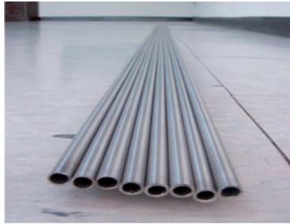
FIG. 11. HT9 cladding tubes.
