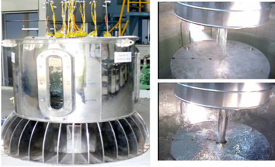
FIG. 3. Grid plate melt through tests.
