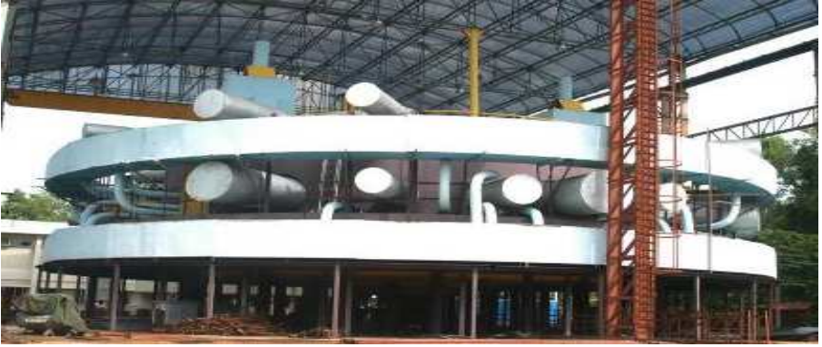
FIG. 10. Full scale top shield layout mock-up.
