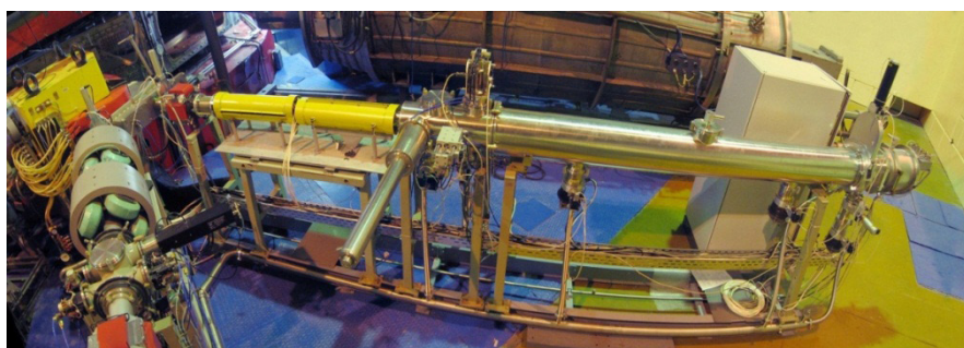
FIG. C-1. Development of a new ion beamline for radiation hardness testing of electronic devices at the U400M cyclotron facility in the Joint Institute for Nuclear Research (Russian Federation).
