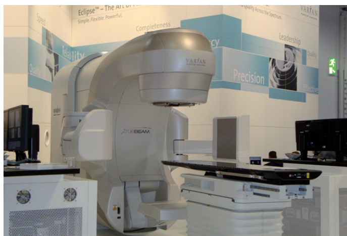
FIG. E-1. A modern medical linear accelerator equipped for IGRT. This device enables increased radiotherapy precision by frequently imaging the target and/or healthy tissues just before treatment and acting on these images to adapt the radiation target.
