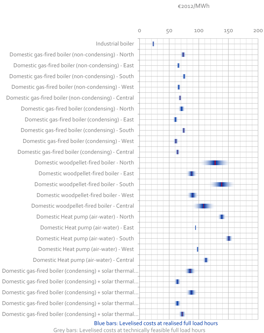
Figure 3-16: Levelised cost of heat in the EU28 for various technologies in the EU28
